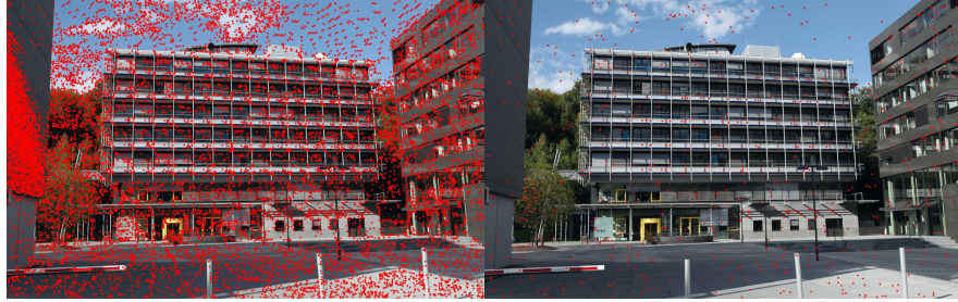
Figure 1.2: Left: all extracted image features ( n=15986 ). Right: pre-selected set of features.
